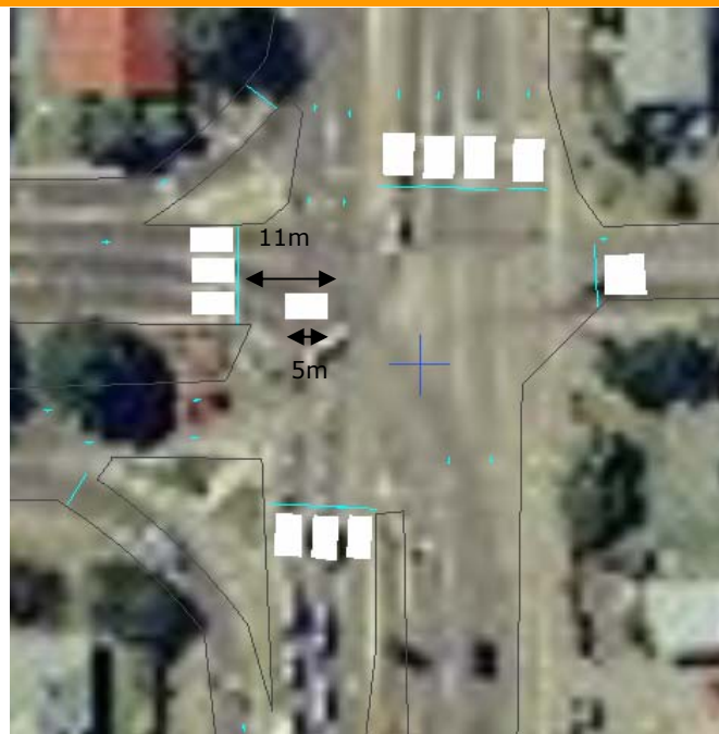
Figure 9: Example Detector Layout at Intersection
