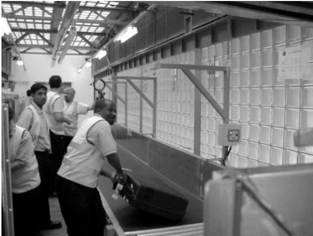
Figure 5-32. The bag is scanned at the platform level and loaded into a container.
