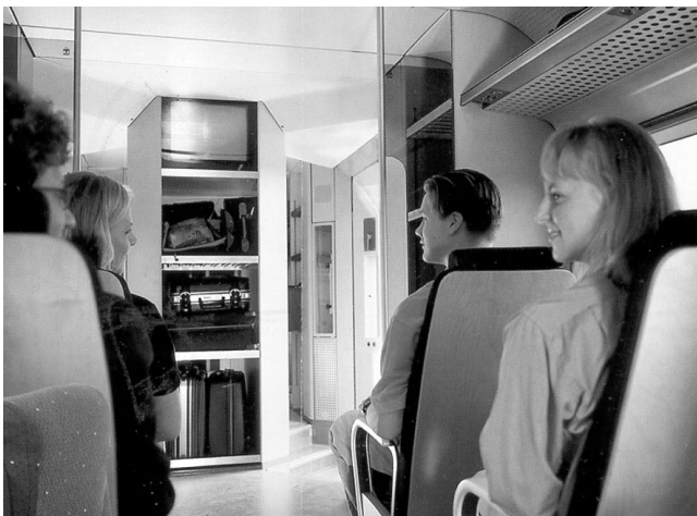
Figure 5-44. All seats face the baggage-storage racks on the Oslo Airport Express trains.
