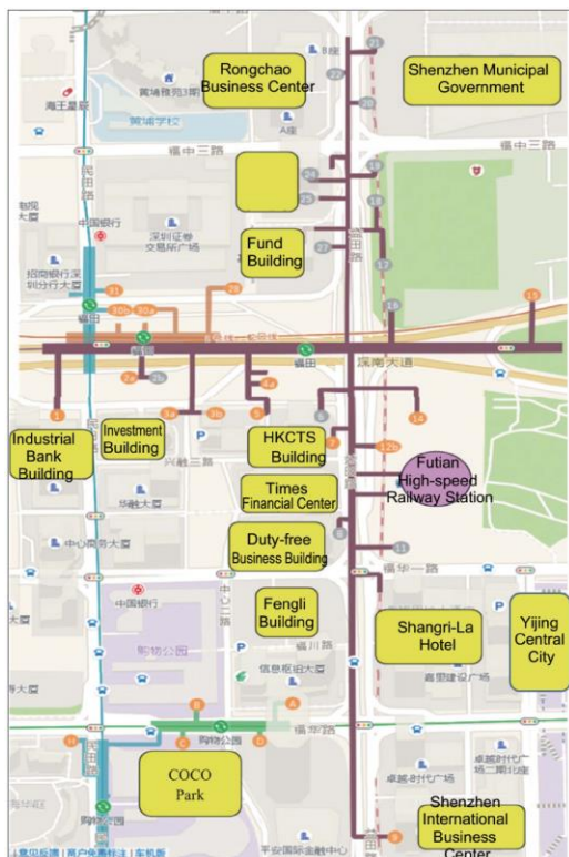
Figure 7 Passages distribution around Shenzhen Futian railway hub
