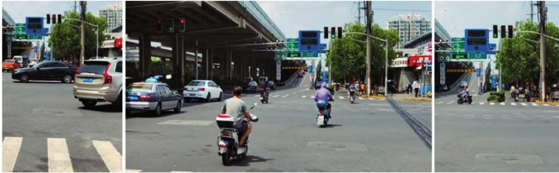
Figure 6 Arrow signal for right-turn vehicles
