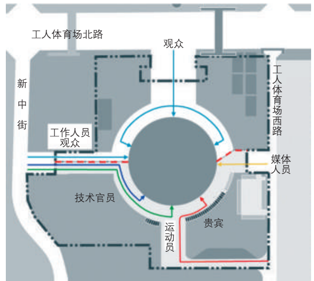
图4 工人体育场不同群体的组织流线图 Fig.4 Diagram of moving paths for different groups at the Worker's Gymnasium
