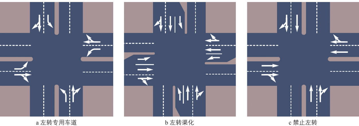
图2 双向道路网络的交叉口配置 Fig.2 Intersection Configurations for Two-Way Networks with: (A) Left-Turn Lanes, (B) Left-Turn Pockets, and (C) Banned Left Turns
