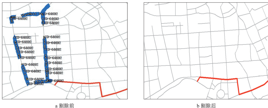
图6 单车辆“伪面”剔除 Fig.6 Removal of single-bus “invalid buffer”
