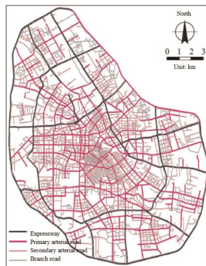
Figure 5 Roadway classification in Tianjin
