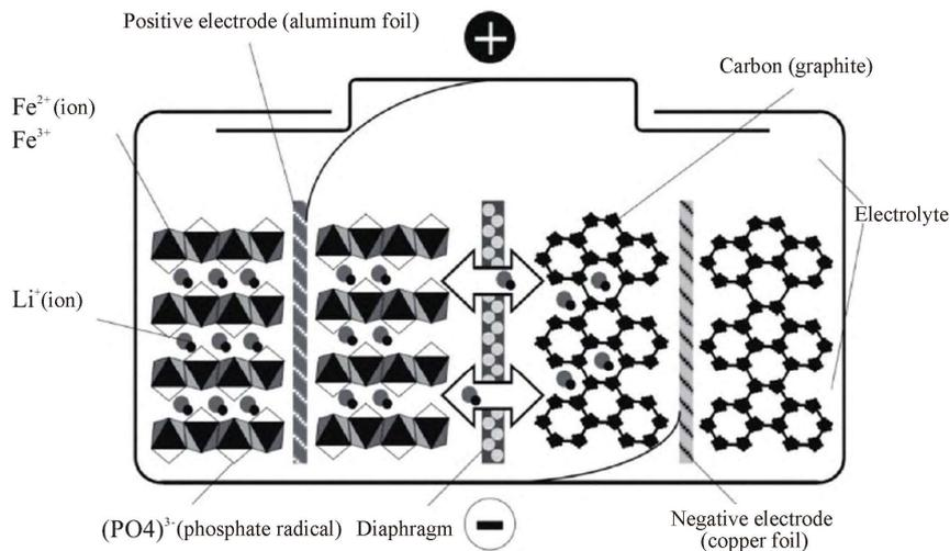
Fig. 6 Internal structure of LiFePO<sub>4</sub> battery
