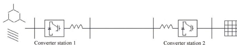
Fig. 5 Two terminal flexible DC transmission system
