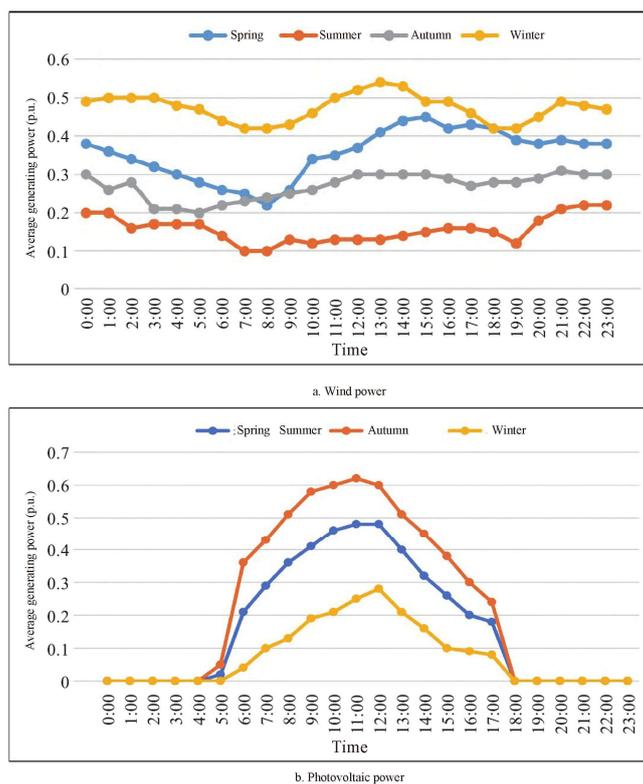
**Fig. 3** Hourly output of wind and photovoltaic power generation by season in North China
