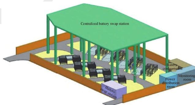
**Fig. 1** Conceptual design of centralized battery swap stations
