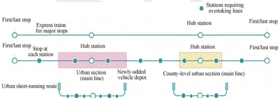
**Fig. 12** Organization mode of rail transit lines with urban rail transit replaced by metropolitan area rail transit
