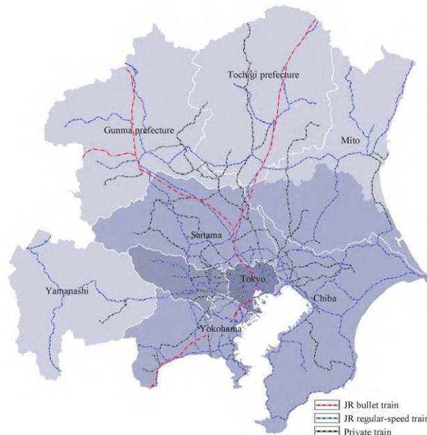
**Fig. 2** Layout of multi-level rail transit network in Tokyo Metropolitan Area
