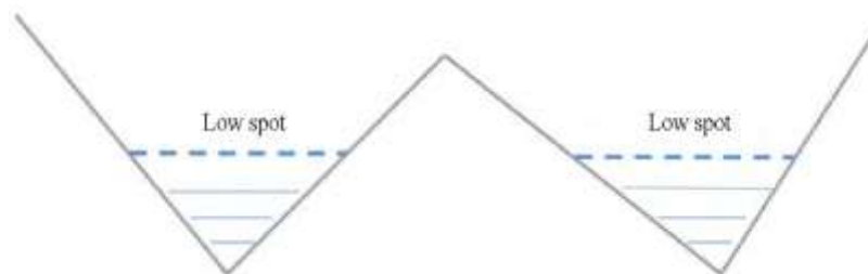
Fig. 13 Illustration of longitudinal slope of serrated roads
