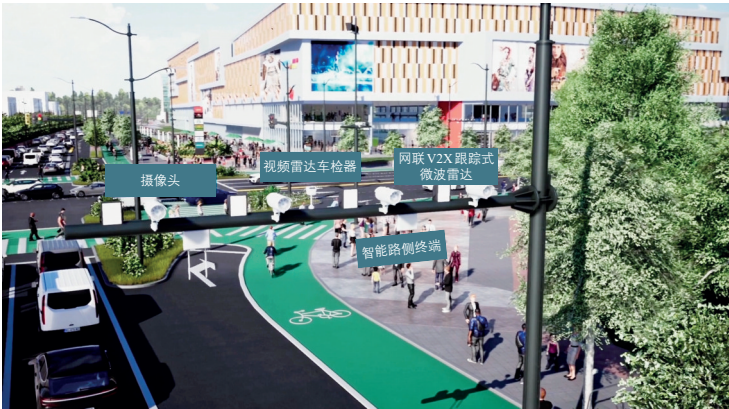
图2 全息交叉口设备布置示意 Fig.2 Layout illustration of holographic intersection equipment
