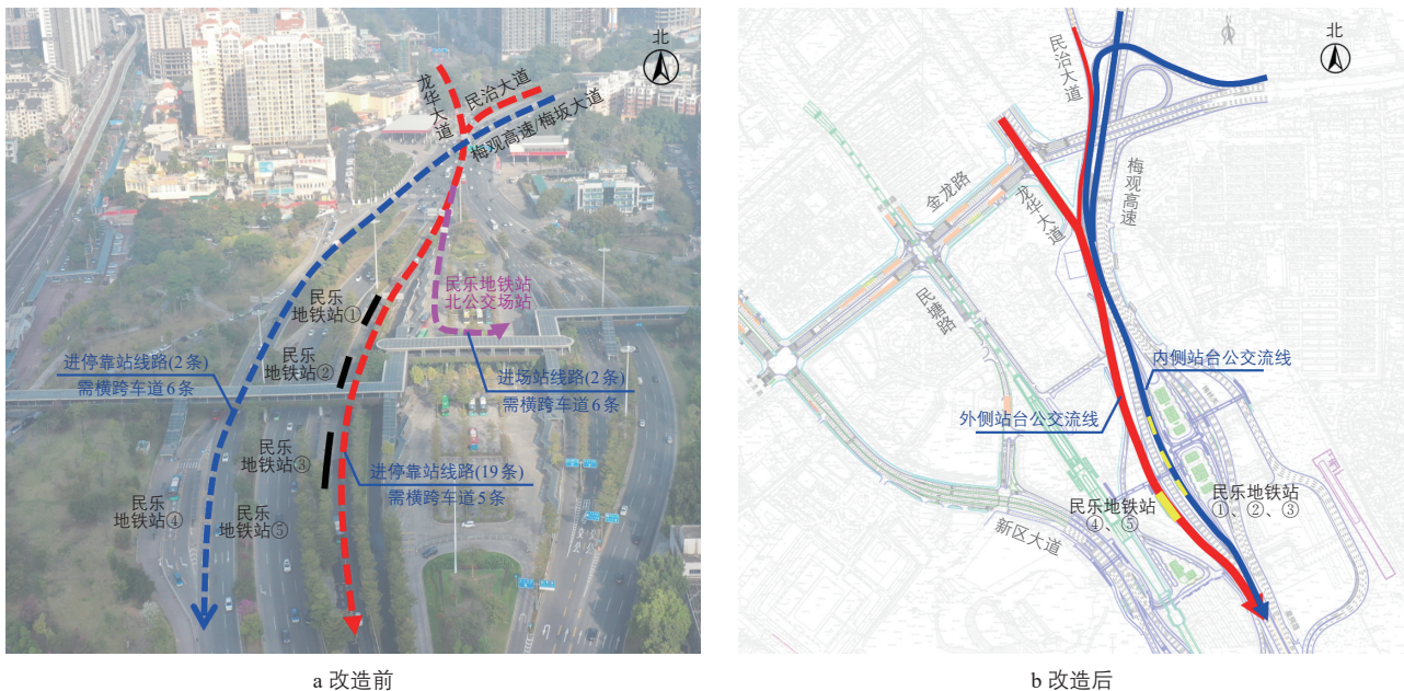
图11 公共汽电车流线优化对比 Fig.11 Comparison of transit bus and trolleybus route optimization
