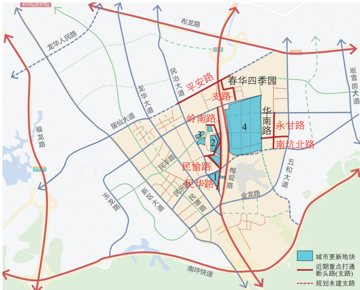
图10 道路微循环通道完善方案 Fig.10 Improvement plan for micro-circulation passages
