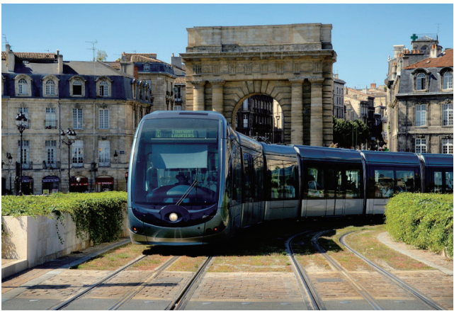
图 2 采用第三轨供电的现代有轨电车 Fig.2 Modern trams powered by the third track
